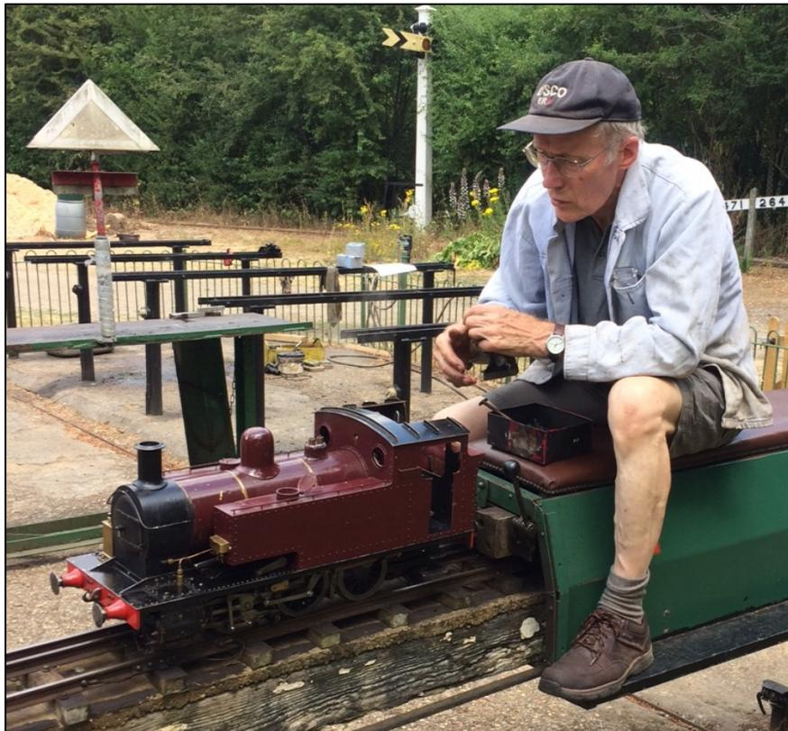
NLSME Club loco "*Butch*" on first run after significant repair undertaken by Mike F. Loco features a new copper (welded) boiler, grate and ash pan.
